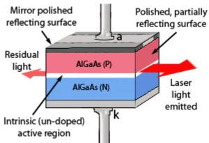
Fig. 2.6.2. Laser Diode Construction
