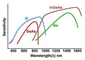
Fig.2.7.13 Relative Sensitivity of Photodiode Semiconductors
