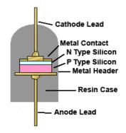
Figure 2.1.2. Silicon Rectifier Construction
