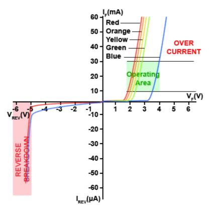
Figure 2.5.8. LED Characteristics Compared
