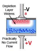
Fig 2.0.6 Diode Reverse Biased
