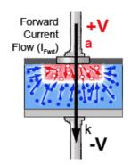
Fig 2.0.5 Diode Forward Conduction
