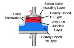
Figure 2.4.1. Zener Diode Construction
