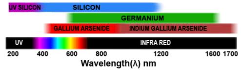
Fig. 2.7.10 Approximate Wavelength Ranges of Common Photodiode Materials
