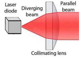
Fig. 2.6.8 Collimating Lens
