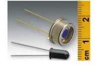
Fig. 2.7.2 Photoconductive diode
