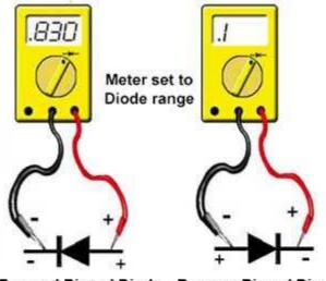
Forward Biased Diode Measures About 500Ω to1KΩ
