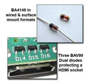
**Figure 2.3.1. Small Signal Diodes**
