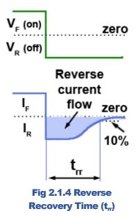
If a reverse voltage  $(V_R)$  is now suddenly applied, as shown in Fig. 2.1.4, the diode should be turned off, but instead of the current through the diode falling instantly to zero, a reverse current  $(I_R)$  is set up as these minority carriers are attracted back across the junction (holes back into the P layer and electrons back into the N layer). This reverse current will continue to flow, until all these charge carriers return to their natural side of the junction.
