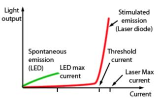
Fig. 2.6.5. Comparison between a LED and a Laser diode
