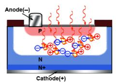
Fig. 2.7.4 Photons Create Electron/Hole Pairs
