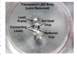
Figure 2.5.3. LED Construction (Top View)
