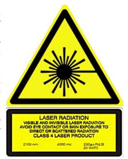
Fig. 2.6.9 Typical Laser Warning Stickers
