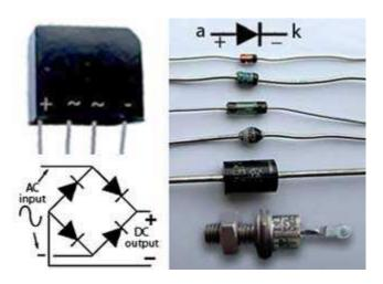
Fig. 2.8.4 Diode Polarity Markings.
