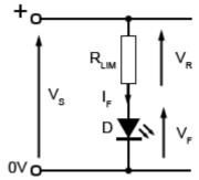
Figure 2.5.9. LED Current Limiting Resistor
