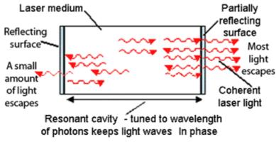
Fig. 2.6.4. The Resonant Cavity
