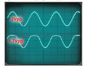
Figure 2.3.6. Clipping a 2Vpp Sine Wave
