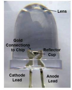
Figure 2.5.2. LED Construction (Side View)
