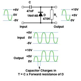
Capacitor discharges in  $T = C \times R_1$
