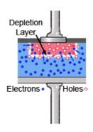
Fig 2.0.4 Diode Depletion Layer
