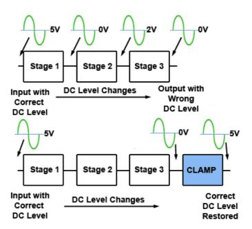
Figure 2.3.7. Clamping or DC Restoration
