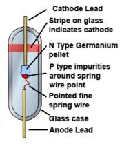
Figure 2.2.3. Germanium Point Contact Diode
