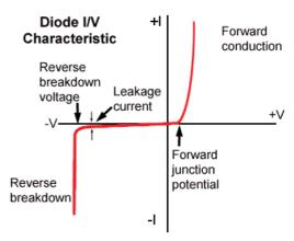
Fig 2.0.7. Typical Diode I/V Characteristic
