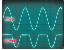
Figure 2.3.5. Clipping a 20Vpp Sine Wave
