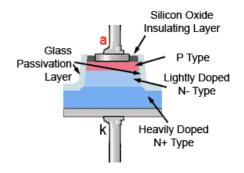
Figure 2.3.3. Simple Mesa Diode
