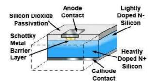
Figure 2.2.2. Small Signal Schottky Diode
