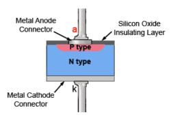
Figure 2.3.2. Simple Planar Diode
