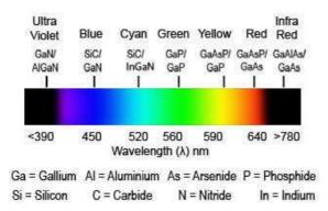
The more energy the electrons lose in this process, the higher the frequency (and the shorter the wavelength) of the light produced. Fig. 2.5.4 illustrates the different combinations of semiconductor materials used to produce light of different colours.
